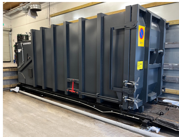
The sturdy scale platform is designed for demanding conditions and installed beneath the waste compactor.
